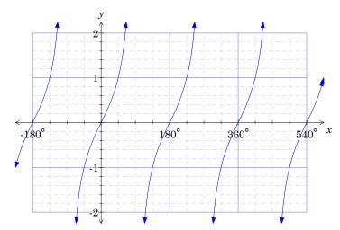
10. Transformations are the same as those for sine and cosine. Note that the a value can be determined by looking at the vertical movement required to move to the right from a point of inflection to a point halfway to the asymptote. For example, the graph below shows  $y = 2 \tan x$ :
